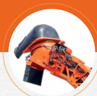
SECONDARY EXTRACTOR HOOD
